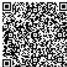
Figure 6 - Example of QR code [30,162mm] e [129 characters] (Size=2, ECC=M, Margin= 2 (0,25cm), Module[version]=9 -> 53x53)
