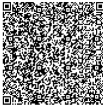
Figure 1 – Example of QR code [47,096 mm] and [452 characters] (Size=2, ECC=M, Margin= 2 (0.25 cm), Module[version]=17 -> 85x85)
