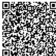
Figure 4 – Example of QR code [30,162 mm] and [116 characters] (Size=2, ECC=M, Margin= 2 (0.25 cm), Module[version]=9 -> 53x53)
