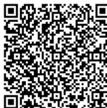
Figure 7 - Example of QR code [30,162mm] e [150 characters] (Size=2, ECC=M, Margin= 2 (0,25cm), Module[version]=9 -> 53x53)
