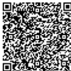
Figure 3 – Example of QR code [32,279 mm] and [209 characters] (Size=2, ECC=M, Margin= 2 (0.25 cm), Module[version]=10 -> 57x57)
