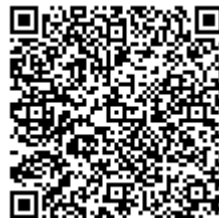
Figure 5 – Example of QR code [30,162mm] e [136 characters] (Size=2, ECC=M, Margin= 2 (0,25cm), Module[version]=9 -> 53x53)
